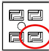
2. Set the Fan Limit Control to Manual (Push the white button in). The blower should start immediately. If so, go to step 10
