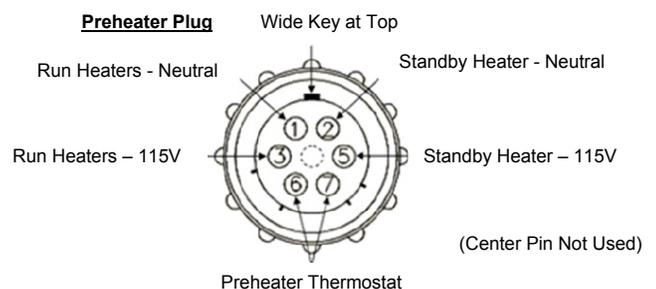
If any of these tests fail, the preheater will need to be replaced.
