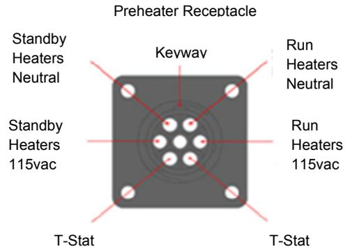
6. If the tests in step 4 and 5 are successful, plug the preheater into the receptacle and allow the preheater to heat up. After 30 minutes, the standby PTC should have heated the oil to the point where the preheater thermostat should have closed. Note: If the room temperature is below 50°F, allow additional time.
