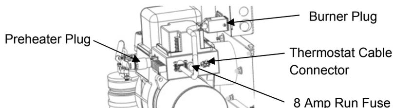
4. Disconnect the preheater plug. Allow the preheater to cool, and check the following with the digital multimeter:
